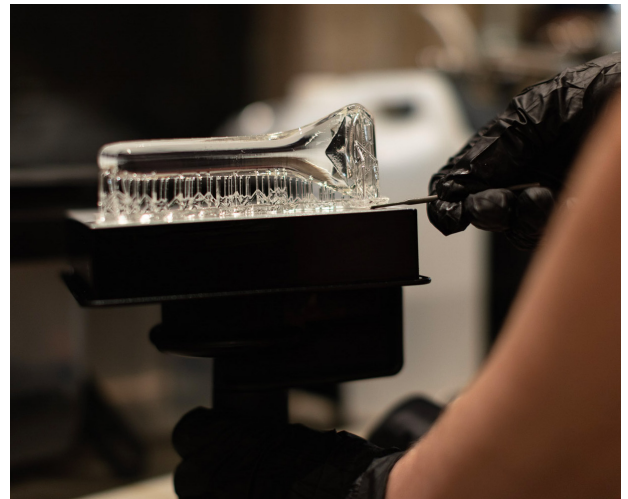
Clear resin 3D prototype on the build platform of the Formlabs Form 3 3D printer
